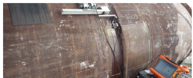
Detection of stage 1 HTHA ©BP Products North America
