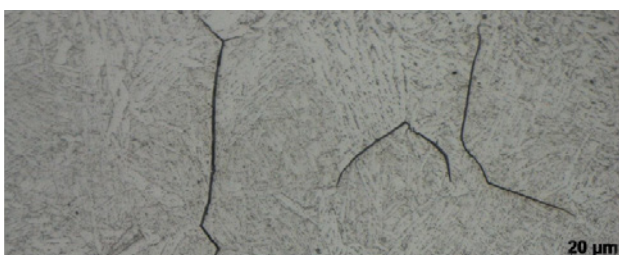
HTHA cracks near the backwall
